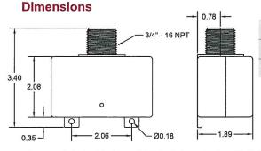
**DITEK's DTK-HW Series** of surge protective devices are designed and manufactured to meet the standards of the life safety industry. These compact, parallel-mount SPD's are available for 120V, 240V and 120/240V systems; and are widely used to protect fire alarm panels and other dedicated branch circuit loads. Their small footprint enables installation in a variety of locations.
